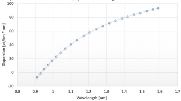
Chromatic dispersion characteristics of nonlinear fiber, dependence on wavelength:
