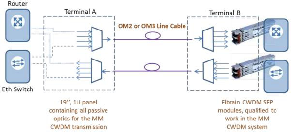
Multimode CWDM transmission system – application diagram
