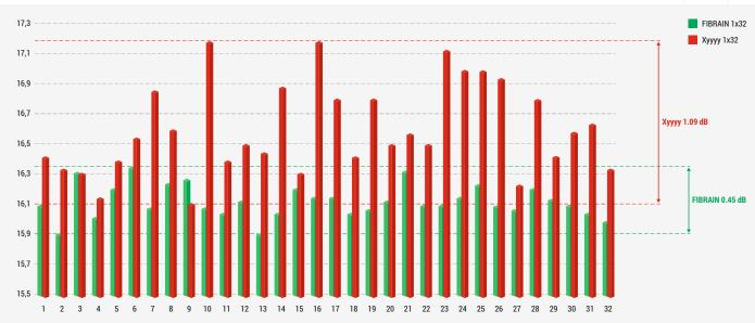
FIGURE 3 – Loss uniformity of 1x32 FIBRAIN - and Xyyyy-branded splitters
