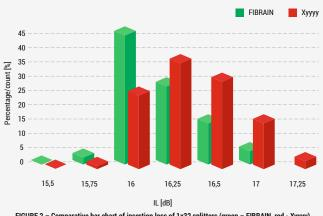
FIGURE 2 - Comparative bar chart of insertion loss of 1x32 splitters (green - FIBRAIN, red - Xyyyy)
