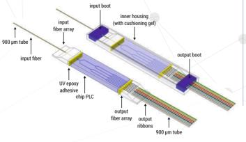
FIGURE 1 - Components of a PLC splitter
